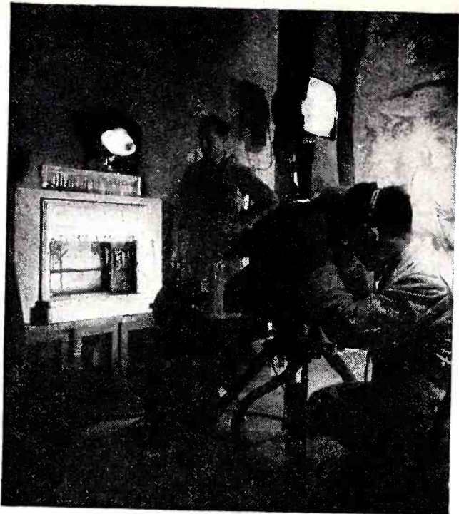
Above—The miniature stage and curtains are viewed by a television camera. This image is broadcast as a preliminary to a television program, the raising of the curtain being the opening feature. When the curtain is up the operator switches over to another camera focused on the "live" scene.
