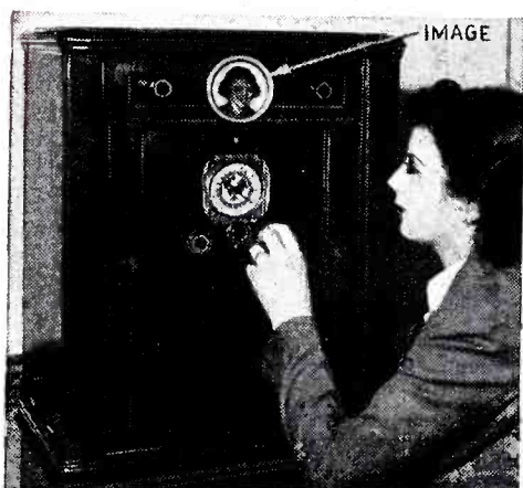
First 441-line television receiver offered for sale to American public. It uses 14 tubes.
